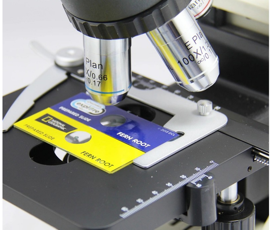
Mechanical Stage Size 145×140mm Travel Range 76×52mm
